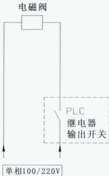
电磁阀 Electromagnetic valve
